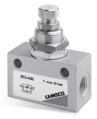
The undirectional flow controllers are equipped with M5 [10-32 UNF], 1/8" and 1/4" ports, each of which is available with two different types of adjustment (see diagrams). They are used mainly for controlling the speed of cylinders. They may be mounted on control panels or cylinders, as required.
