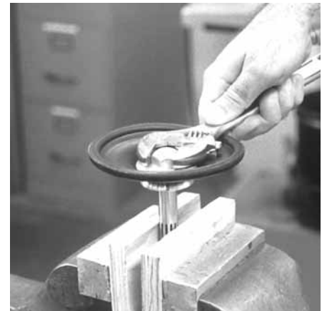
Step 12. Figure 12 To remove the diaphragm assembly from the shaft, secure shaft with soft jaws (a vise fitted with plywood or other suitable material) to ensure shaft is not nicked, scratched, or gouged. Using an adjustable wrench, remove diaphragm assembly from shaft. Inspect all parts for wear and replace with genuine Wilden parts if necessary.
