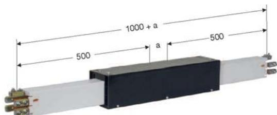
The Expansion sections are required to compensate the different expansions between copper conductors and steel- or concrete structures, in varying temperatures without interrupting electrical power.
