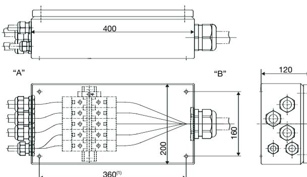
Electrical connection with customer supplied cable shoes. Clamping range 16-95 sqmm.
