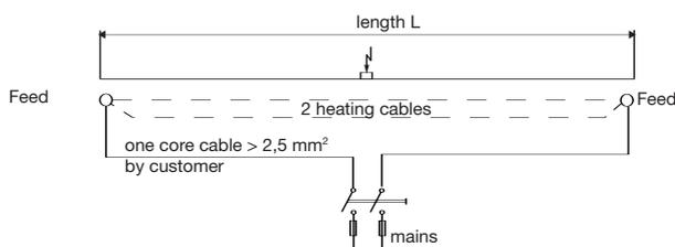
Switch gear assembly and temperature control unit as per customers inquiry. Fuses, cables etc. have to be provided by the customer.
