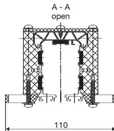
By opening and closing the sliders at the bottom of the powerail housing the collector can be mounted and demounted easily.
