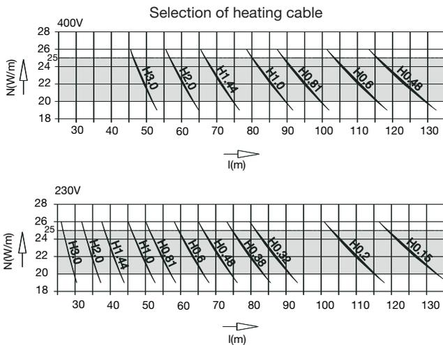
**Heating capacity [Watt/m]:**  $N' = \frac{U^2}{R \cdot L^2}$
